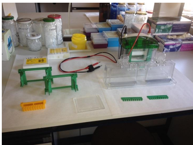
Figure 3. Components of a vertical electrophoresis cell (BioRad) used in our experiments
