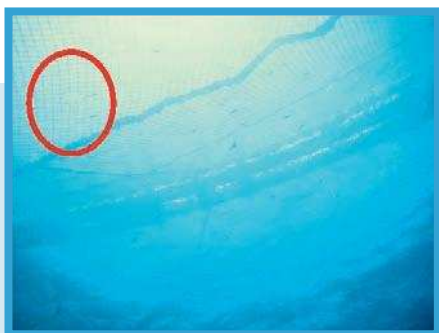
FIGURA 14.5. Rotura de red (Global Aquafish).
