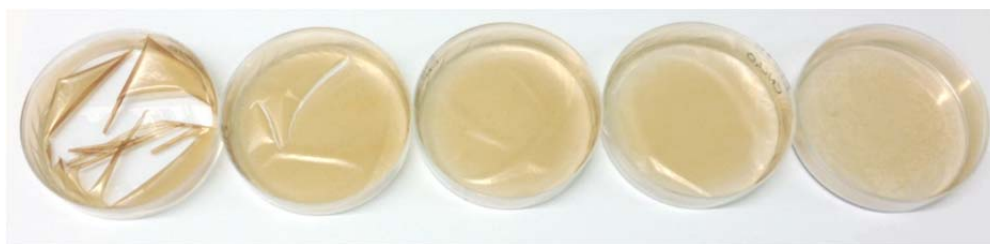
Figure 2. Film formation with a CNC content of 10%, 20%, 30%, 40% and 50%, from the left to the right.
