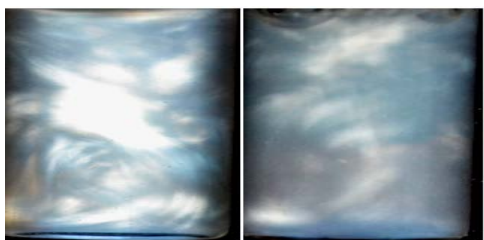
Figure 5. Flow birefringence of succinylated cellulose nanofiber suspension in DMSO (left) and water (right).
