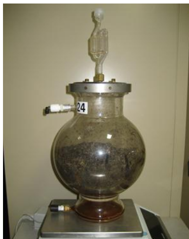
Figure 1. Anaerobic Biopulping Apparatus
