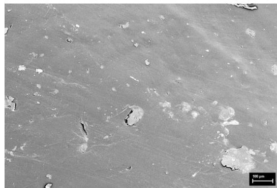
Figure 4: SEM image of CNC-AO 4/PP compound, darker matrix is PP, lighter areas are CNC-AO 4.
