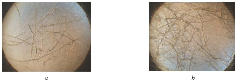
Figure 1 – The microphotographs of films obtained by a digital microscope. The cellulose fibers introduced into the composition: a – 15 %; b – 25 %
