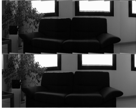
Figure 3.1: Intensity jumps between successive images caused by automatic camera gain. Applying linear blending solves the problem.
