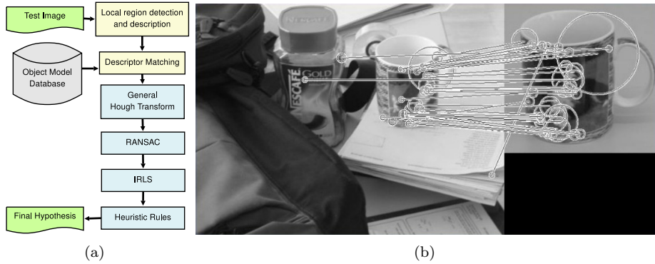
Figure 5.1: (a) Diagram of the modified SIFT object recognition method. (b) Matching stage in the SIFT object recognition method.
