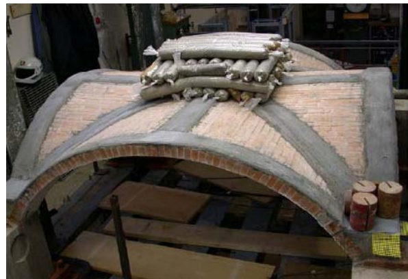
Figure 2.7. FRP strengthening of a masonry cross vault.
