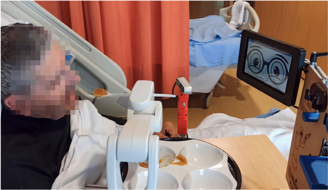
Prototype of a robotic feeding system, co-designed by the Institut de Robòtica i Informàtica Industrial (CSIC-UPC) and the Parc Sanitari Pere Virgili in Barcelona
