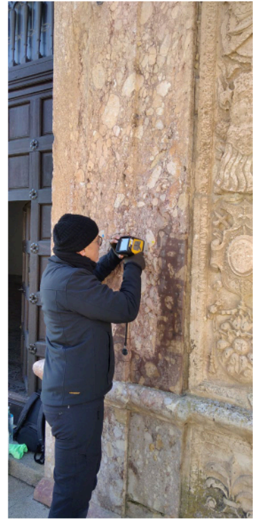
In situ characterisation using portable X-ray fluorescence equipment of the conglomerate ashlar of Espejón (Soria), used in the Renaissance doorway of the palace of the Counts of Miranda (Peñaranda de Duero, Burgos). / VIRGINIA GARCÍA-ENTERO
