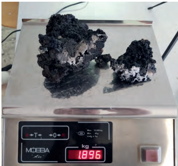
Figure 8: Weighing of the resulting experimental bloom. Note the typical spongy appearance, with the porosity filled with all sorts of melting slags. Image: © B. Asmus.
