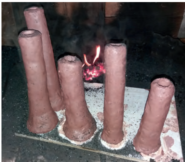
Figure 2. Tuyères of different sizes, drying in the forge (Foto: T. Mink).
