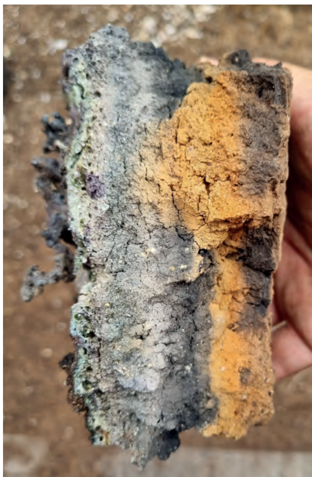
Figure 4: This image show a piece of furnace wall, that was vitrified during the smelting process in its inner regions. Note the thickness of the slag adhering to the walls, as well as the heat affected zone of the wall. The grey clay indicates strongly reducing atmosphere, which reduced the iron oxides in the clay to FeO. Image: © B. Asmus.
