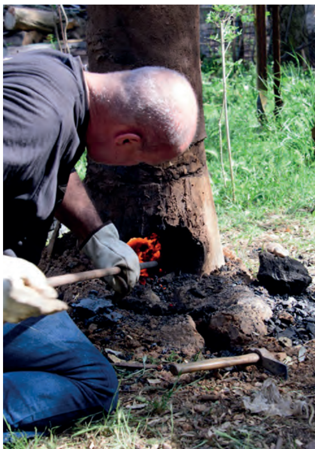
Figure 9. Bloom extraction during a course I offered at the Blacksmithing school of Ramón Recuero (Toledo) (Foto: courtesy of T. Mink).
