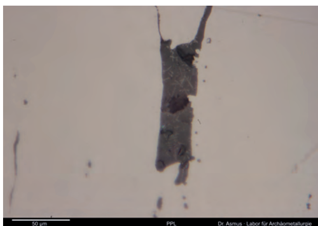
Figure 14: High magnification of a larger slag inclusion within the weld: Wüstite dendrites within the slag. Image: © B. Asmus.
