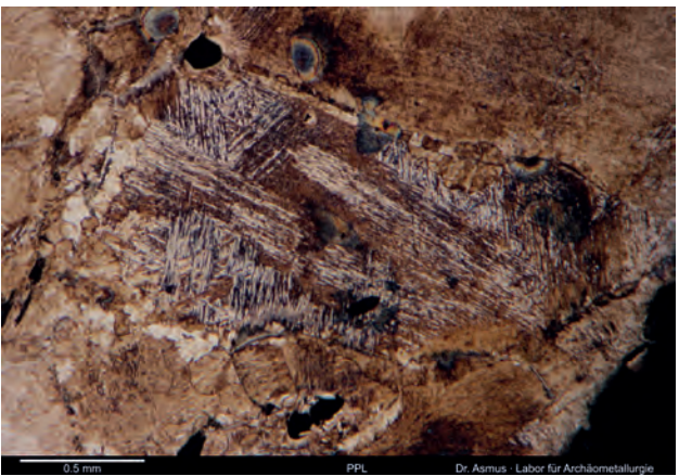
Figure 11: Bloom, etched cross section with 2% Nital solution. Bainite, a structure formed when cooling low carbon steels not fast enough to form martensite, but faster than to form pearlite. Image: © B. Asmus.
