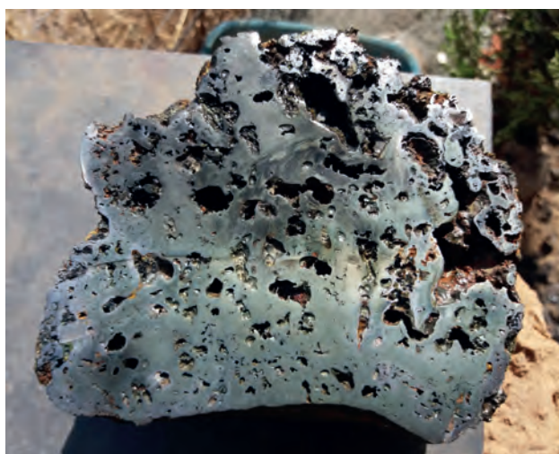
Figure 8. Example of a bloom that has grown below the tuyère. The deformation that the air flow has created on it is clearly visible. The direction of the air stream is visible as it hit from the left side and pushed the iron particles to the right (Foto: T. Mink).
