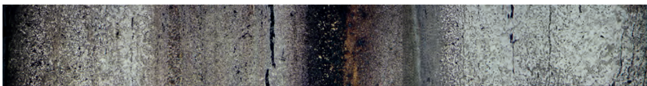
Figure 15: A composite of six micrographs. Total width of the sample is 8.5 mm. Etched Nital 2%. Note the very heterogeneous layered composition. The highest carbon content is in the centre, where the steel has a eutectoid composition. The largest part of the sample has a much lower low carbon content, with areas of almost pure ferritic composition. Image: © B. Asmus.
