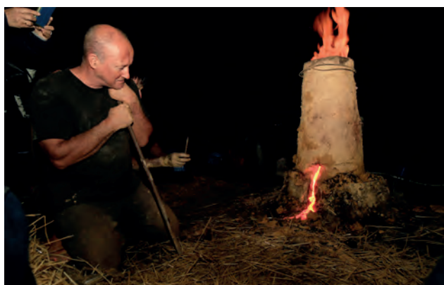
Figure 7. Tapping with a good slag output from the furnace (Foto: Jose Salgado).
