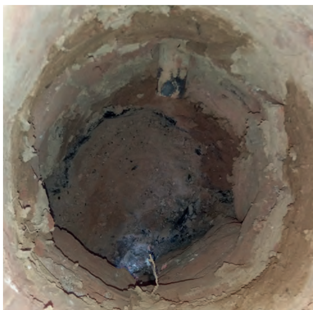
Figure 3. Interior of a furnace that was built at the blacksmiths' meeting in Estada (Huesca, Spain). The tuyère is visible at the top of the image. This furnace did not have an interior coating, due to the lack of time for its construction (only two days). Although this greatly reduced the smelting performance, the result was still satisfactory (Foto: T. Mink).
