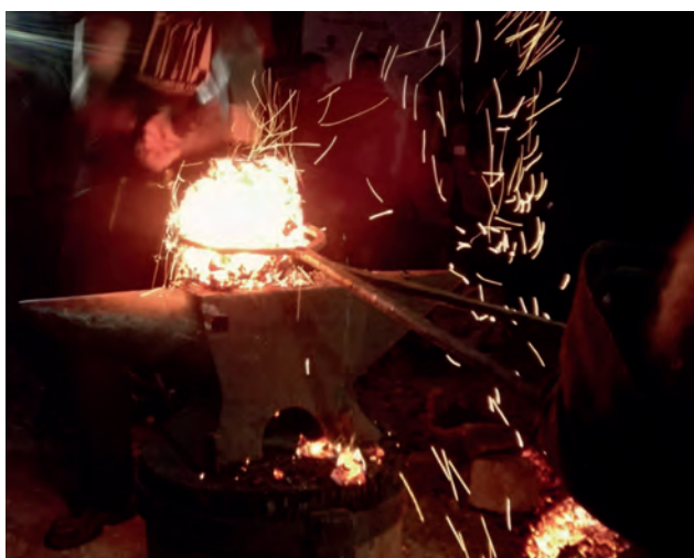
Figure 10. Once the bloom has been removed from the furnace, an initial refinement can be carried out by taking advantage that it is hot enough. This is here done on an anvil, although a wooden log would be ideal to keep the welding temperature (Foto: T. Mink).
