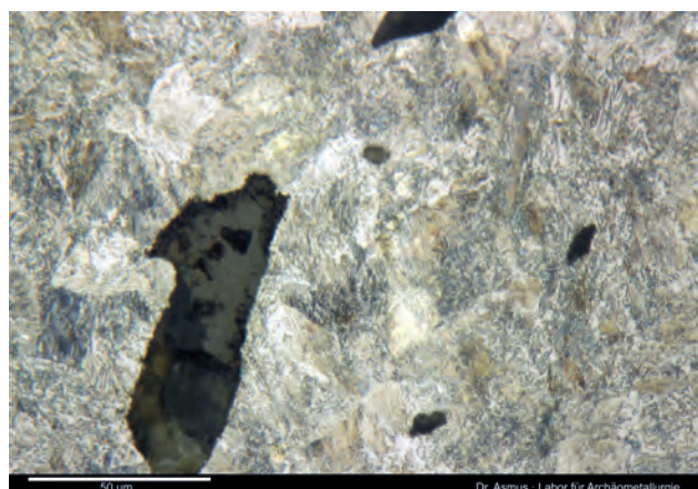
Figure 20: Steel chisel from Rocha do Vigio, etched 2% Nital. This section shows a near eutectoid composition. There is almost only pearlite. Also there is a large slag inclusion. This section represents those regions of the chisel with the highest carbon content. Image: © B. Asmus.
