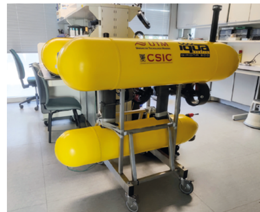
Figure 2. Girona500 AUV model at the facilities of the Unitat de Tecnologia Marina in Barcelona.
