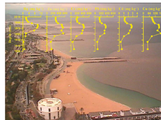
Figure 2. Plumes of turbid and untreated polluted water discharged during extreme rain and flood events on the Barcelona city coast. In yellow, vertical profiles of trace metal concentrations in the sediment showing their historical evolution. (from Palanques et al. 2017).
