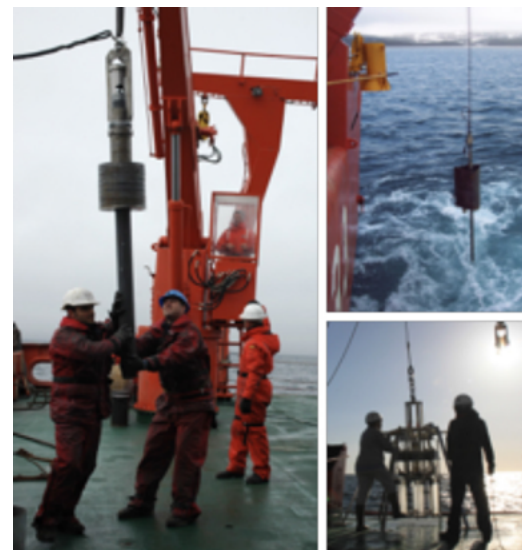
Figure 1. Coring systems of deep-sea sediments: gravity corer (left and top right) and multicorer (bottom right). Images: Unitat de Tecnologia Marina (UTM-CSIC).
