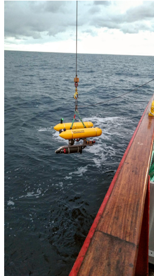
Figure 1. The Girona 500 AUV used to track Norway lobsters ( Nephrops norvegicus ) at 400 m depth in the NW Mediterranean Sea.
